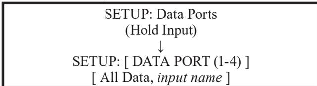
**All Data:** Devices connected to all four data ports will receive the same data from the Remote Control.
