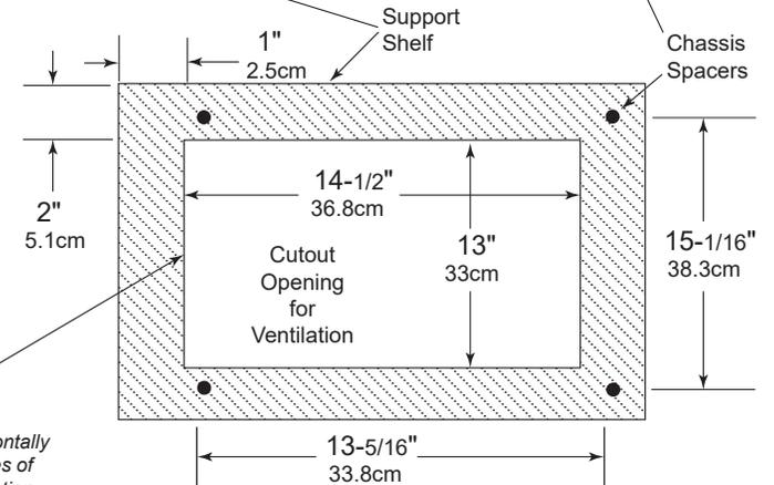
Note: Center the cutout Horizontally on the unit. For purposes of clarity, the above illustration is not drawn to scale.
