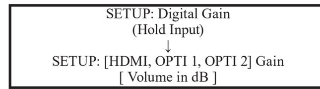
To get more even playback Volume from your connected digital devices, adjust their individual volumes with this Setting. The defaults are +15dB for HDMI and +0dB for Optical.
