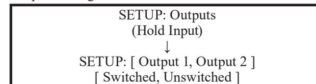
**Switched:** The front panel/Remote Control Output buttons will function as normal, allowing you to toggle On and Off the outputs.
