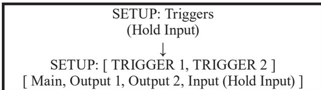
**Main:** An On/Off signal is sent to devices attached to the TRIG 1 and TRIG 2 ports when the MA8950 is turned On or Off.
