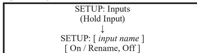
**On / Rename:** The selected Input will be functioning as normal. Hold in the Input Control Knob to enter the Menu to rename the Input\*.
