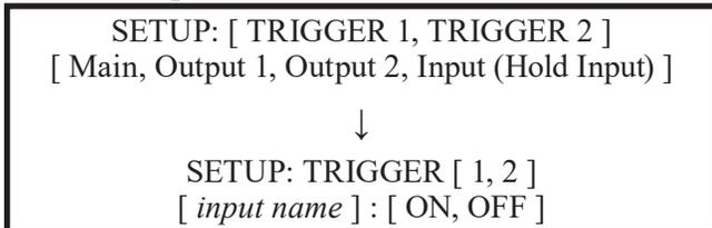
**[ input name ] : ON:** Turns On/Off any devices attached to TRIG 1 or TRIG 2 when the Input is selected on the Main Display during normal use.
